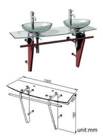
**DESCRIPTION:** 1.Material: Sepetir/BRASS JIS2600 with chrome plated 2.Water-proof coating 3.Level adjustable 4.N.W.: 15 kg 5.Deck: Tempered glass (L)1500x(W)480x15(mm) 6.Washing table for two basins
