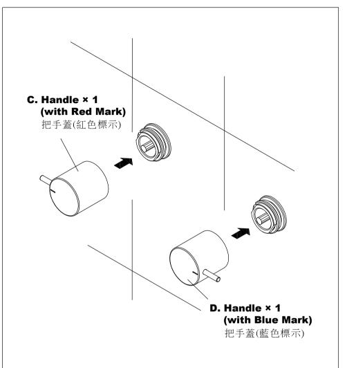
\* Confirm **Hot Valve** and **Cold Valve** have been turned to closed position before install the **Handle**. Press both hot and cold **Handles** onto valve spindles until hear the click sound as the figure shows. 確認冷熱水開關已轉至關水位置。將把手桿保持在水平位置組入中心栓,壓到底之後會有喀噠聲,表示安裝完成。
