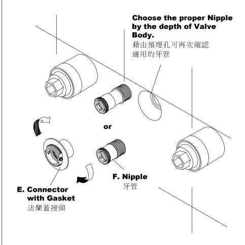
\* Choose proper **Nipple**, apply the pipe compound or thread sealant tape and then screw it to the **Valve Body**. Screw and tighten **Connector with Gasket** to the **Nipple**. In case of forgetting the choosing parts, it could be checked again by the depth of Valve Body. 選擇適合的牙管後,纏上止洩帶鎖入牆內閥體。再將法蘭蓋接頭穿過墊片後鎖入牙管。若不慎忘記選用的零件,可利用預埋孔的深度
