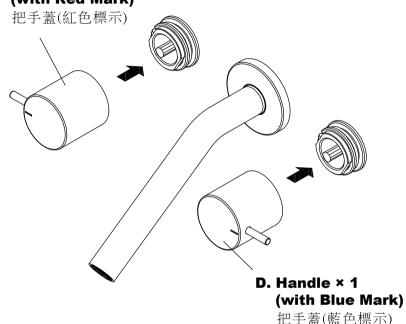
\* Confirm **Hot Valve** and **Cold Valve** have been turned to closed position before install the **Handle**. Press both hot and cold **Handles** onto valve spindles until hear the click sound as the figure shows. 確認冷熱水開關已轉至關水位置。將把手桿保持在水平位置組入中心栓,壓到底之後會有喀噠聲,表示安裝完成。
