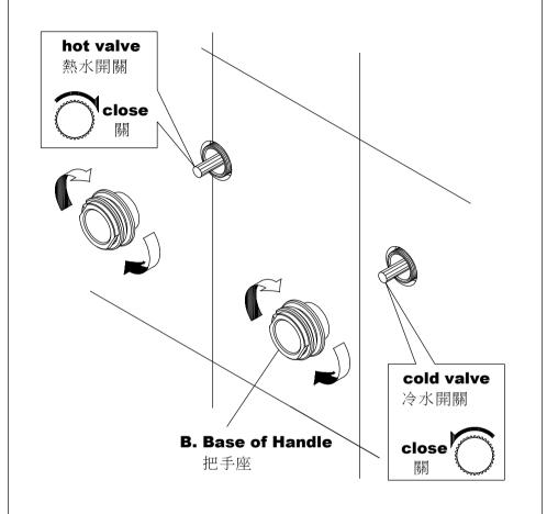
\* Screw the **Base of Handle** to the shanks of **hot and cold valves** till against finished wall.
