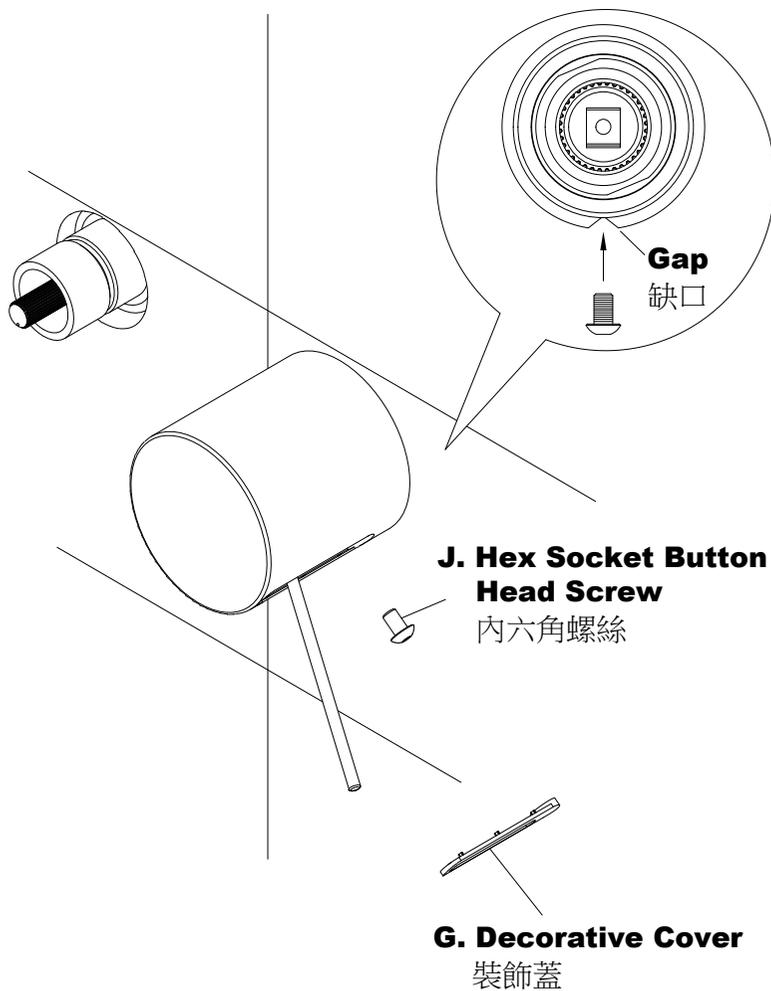
\* Fix the **Handle** to the Base with the **Hex Socket Button Head Screw**, and then add the **Decorative Cover**.
