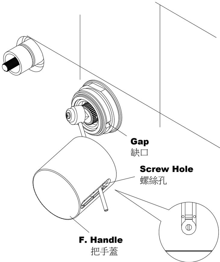
\* Insert the Lever through a hole in the **Handle**. Completely cover the handle base. Aim the screw hole into the gap.
