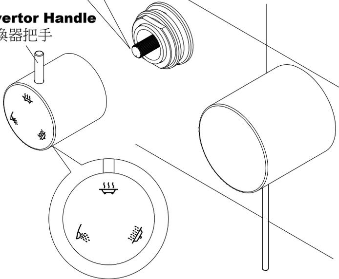
\* Turn the **Divertor Spindle** until the point mark stops at 6 o'clock position. Insert **Divertor Handle** into the spindle. You shall hear a "click" sound.
