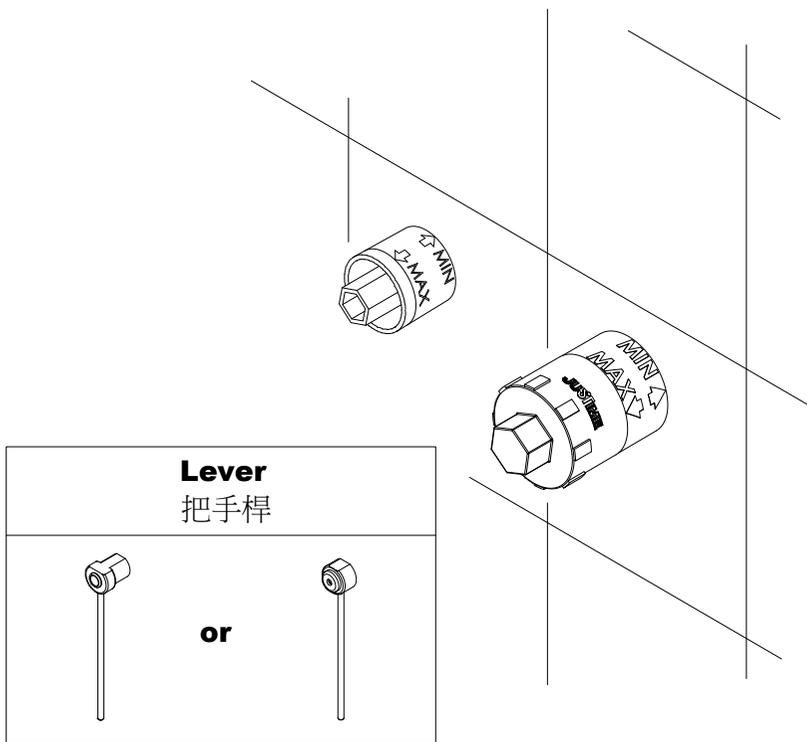
\* Before installing handle, choose the proper **Lever** according to the distance from top of the **Sleeve** to the finished wall.
