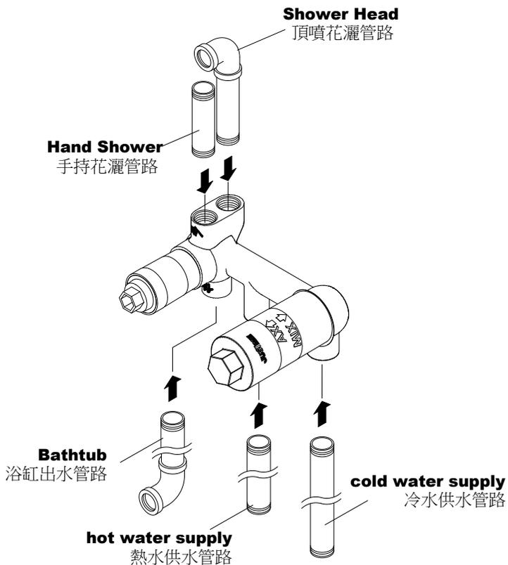
\* Install outlet pipes, hot and cold water supply pipes as figure shows.
