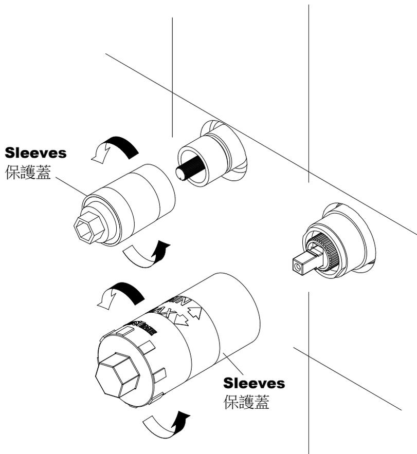
\* Remove the **Sleeves** only when the proper **Lever** was selected.
