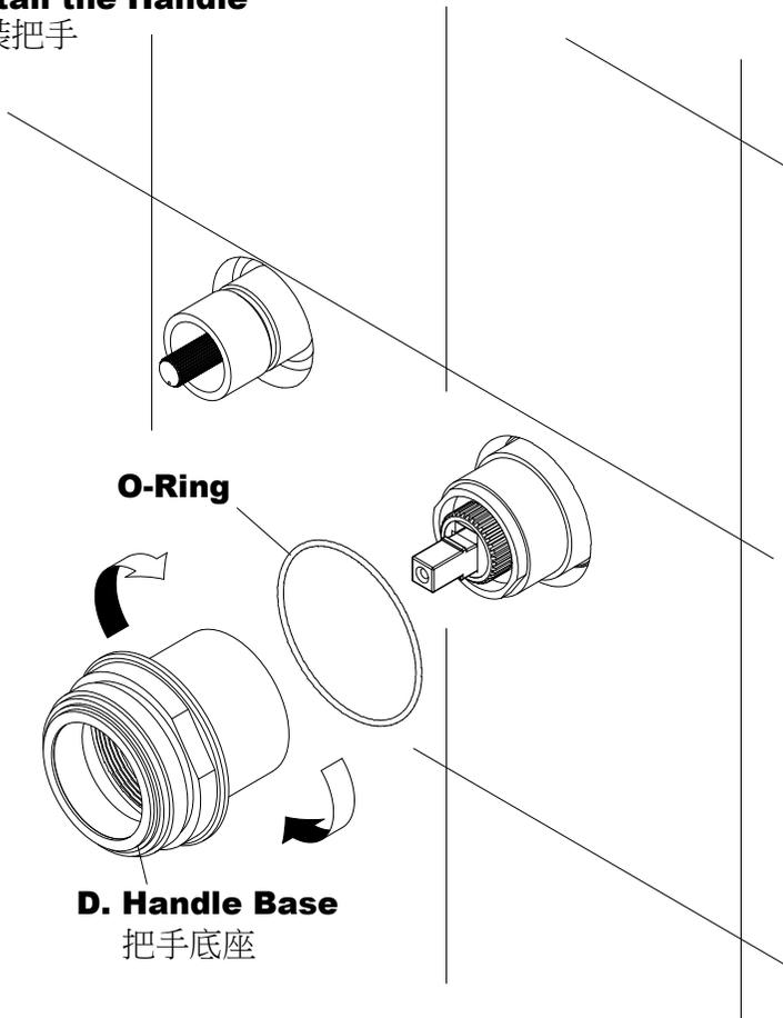
\* Screw in the **Handle Base** with **O-Ring** clockwise to the **Valve Body** and tighten it. Please notice the **O-Ring** has to be placed between base and wall.
