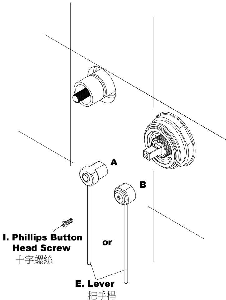
\* Fix the chosen **Lever** to the top of cartridge with **Phillips Button Head Screw**.
