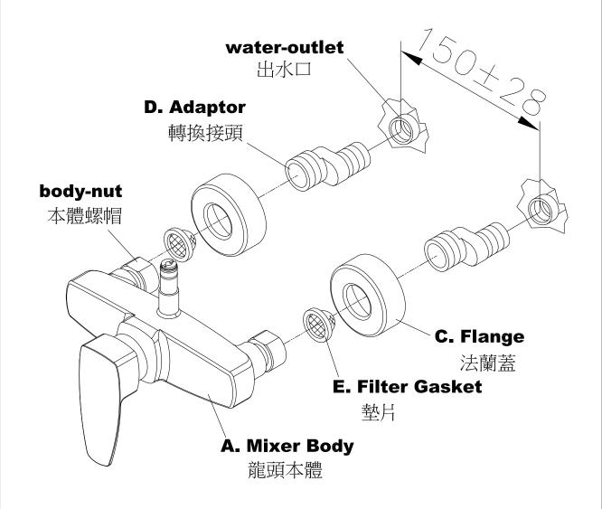
\* Apply pipe compound or thread sealant tape to the thread of **Adaptor** 1/2" end, and screw it into wall water-outlet, meanwhile, adjust the distance between two **Adaptor** 3/4" ends to 150mm for **Mixer Body** connection. Cover **Flange** onto both 3/4" end of **Adaptor**. Insert **Gaskets** into each body-nut, screw the body-nut onto **Adaptor** 3/4" end, and then tighten the nut to well fix.
