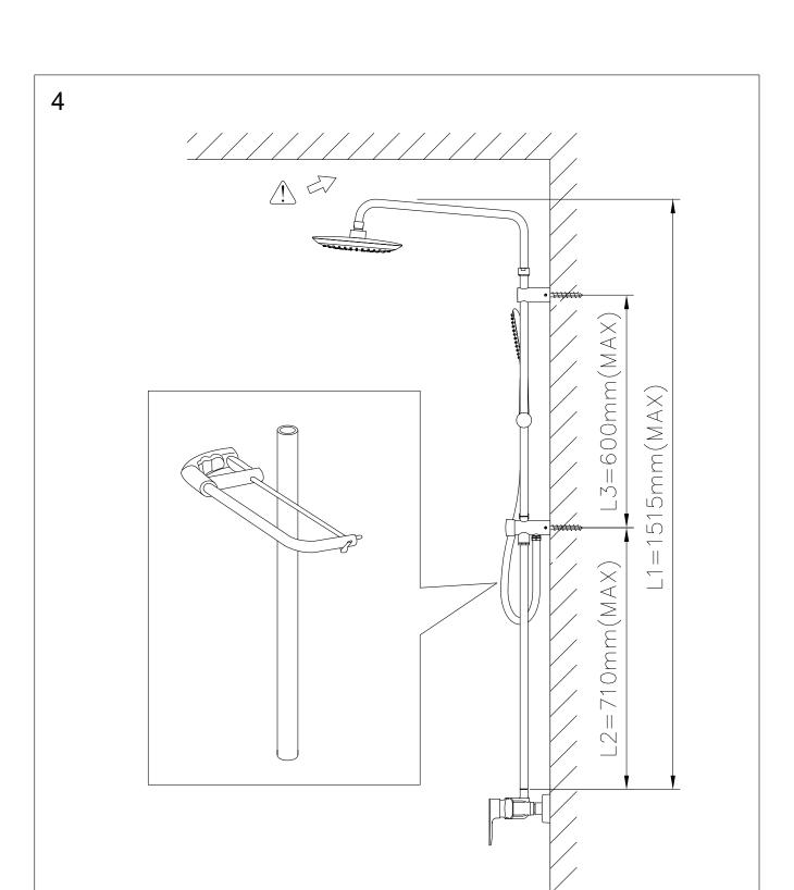
\* WARNING: Reduce the length of L2 if necessary to ensure whole "Rain Shower" can be installed beneath the ceiling.
