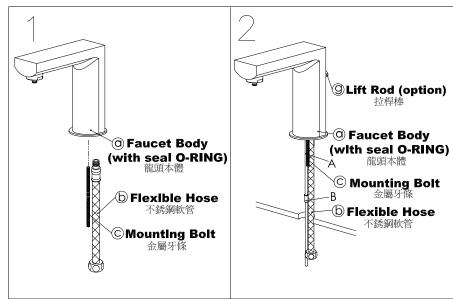
1. Screw Flexible Hoses and Mounting Bolt into Faucet Body (with seal O-RING).
