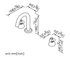
ø60 [2<sup>3</sup>/8] 168 [6<sup>5</sup>8] ø25.4 [1] 196 [7<sup>1</sup>%6] 34 [17/6] 128 [5<sup>1</sup>/16]  $[2^{1}_{4}]$ ø52 [2<sup>1</sup>16] 56 102 [4] 1 1/8-18UNEF 1 1/8-18UNEF G1/2--G1/2 L: 450 [17<sup>1</sup>/16]-E ſſ LG1/2 G1/2\_
