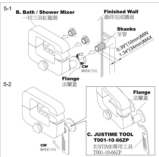
\* For fixing the **Bath / Shower Mixer** Body with the **Shanks**, there should be 10mm~34mm (0.39"~1.34") outside the **Finished Wall**. Then screw the **Flanges** by hands & **JUSTIME Tool T001-10-66ZP** securely against wall.
