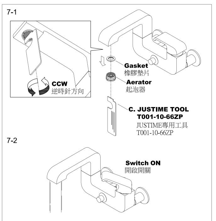
\* Risk of product damage, when finished installation, please disassemble the **Aerator** and **Gasket** counterclockwise with **JUSTIME Tool T001-10-66ZP**, and then fully turn on the hot and cold water valve to run for one minute as first using. After turn off water, please assemble the **Aerator** and **Gasket** with opposite steps as disassembling.
