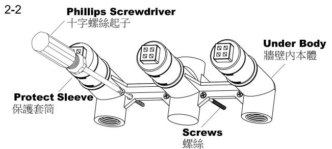
\* Connect hot and cold supplies pipes to the **Under Body**, so they are between 2"(5cm) minmum and 3"(7.6cm) maximum from the finished wall, then fixed the **Under Body** in place with **Serews** or **Pipe Clamps**.
