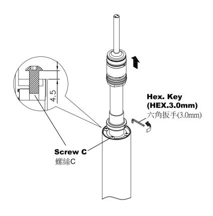
\* Loosen all the **Screw C** and pull up the cartridge spindle slightly. Please DO NOT pull up the cartridge spindle hard for avoiding breaking the braided hoses to cause leaking.
