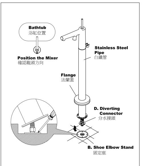
\* Position the **Bath Mixer** to Bathtub before installation, and press the **Diverting Connector** into the **Shoe Elbow Stand** with fingers and tools.
