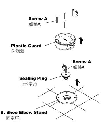
\* Disassemble the **Screw A** of **Plastic Guard**, and remove the **Plastic Guard**. Screw the **Screw A** into the **Sealing Plug** to pull out the **Sealing Plug**.
