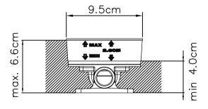
\* The available height from ground to Finished Floor is between 4.0cm and 6.6cm; the marks of plastic guard could be referenced as floor construction.
