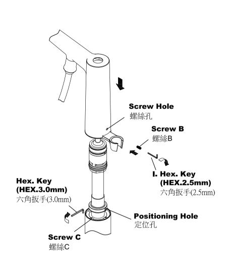
\* Tighten the **Screw C** to fix the cartridge spindle on the stainless steel pipe. Align the **Screw Hole** of **Shell** with the **Positioning Hole**, cover the shell, and then fix with the **Screw B**.
