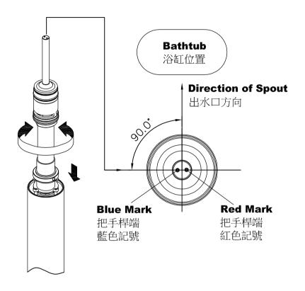
\* There are 60 positions for adjustment in 360 degrees. Use the **Blue** and **Red Marks** on Handle as reference while positioning, and then assemble the cartridge spindle on the stainless steel pipe.
