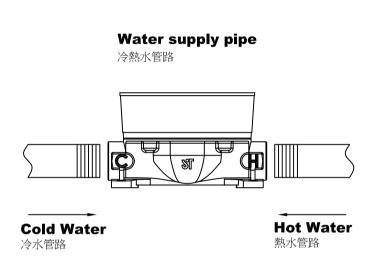
\* Connect the hot and cold water supply as the marks on the **Shoe Elbow Stand**. After finish the installation, please make sure if the connection of hot and cold water supply are same as the marked indication on the **Shoe Elbow Stand**.
