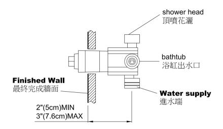
\* Connect hot and cold supplies pipes to the valve body, so they are between 2"(5cm) minmum and 3"(7.6cm) maximum from the finished wall; or keep the distance be 0.4" (1.1cm) to 1.5" (3.7cm) between top of cartridge and **Finished Wall** for necessary conditions.
