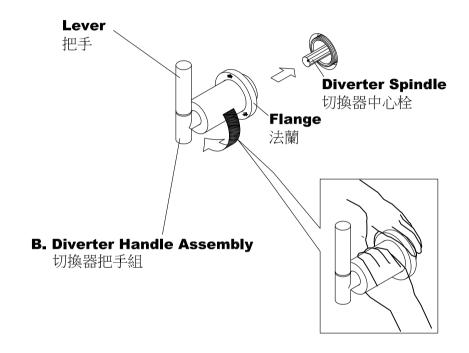
\* Rotate the **Flange** to make the **Rain Shower Sign** be kept on top position. Arrange the **Lever** to be upward, press the **Diverter Handle Assembly** onto the **Diverter Spindle**, and then screw the **Diverter Handle Assembly** by hands till against the finished wall.
