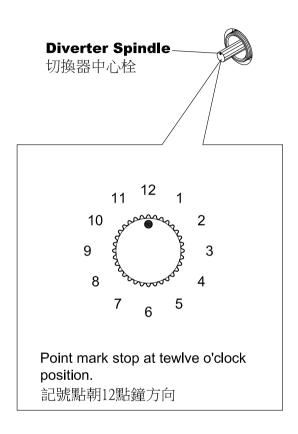
\* Face to the **Diverter Spindle**, and then adjust the **point mark** of **Diverter Spindle** to the tewlve o'clock position.
