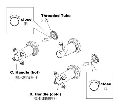
\* Turn **Hot Valve** and **Cold Valve** clockwise to closed position before install the **Handle Assembly**. Press both hot and cold **Handle Assembly** onto valve spindle and securely hand tighten the **Handle Assembly** against finished wall.
