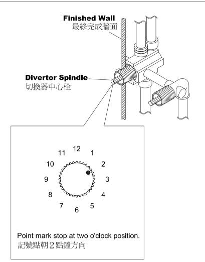
\* Keep the **Mixer Valve** straight ahead of you, then turning the **Divertor Spindle** until the **Point mark** stop at two o'clock position.
