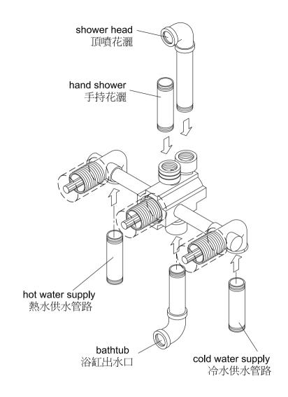
\* Install hot and cold water supply pipes and outlet.
