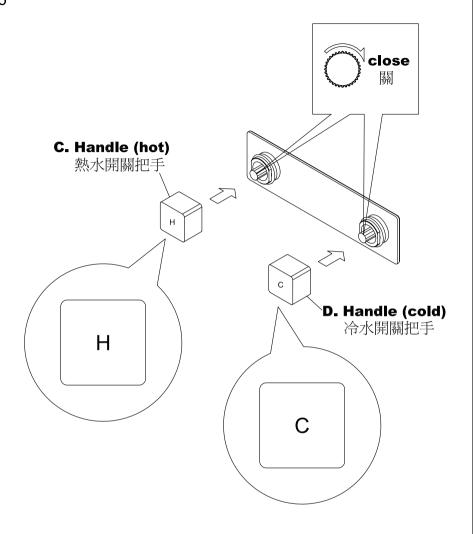
\* Turn **Hot Valve** and **Cold Valve** clockwise to closed position before install the **Handle**. Press both hot and cold **Handle** onto valve spindle until heard a click sound.
